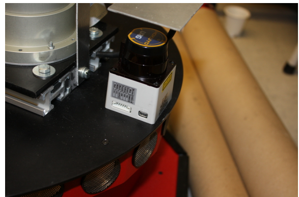
Figure 23: Zoom of correct laser orientation
