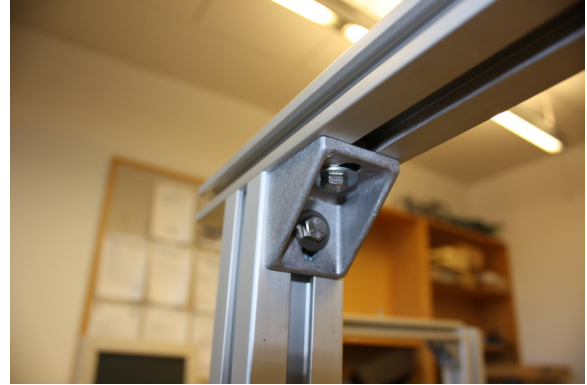
Figure 29: Bracket mounting of top beam
