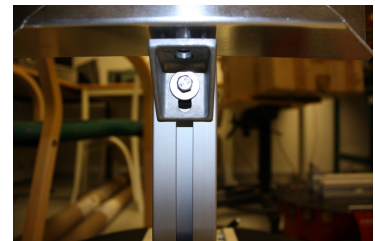
Figure 44: Supporting bracket at bottom of laptop holder
