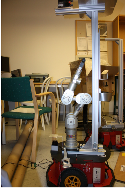
Figure 46: Katana arm mounting
