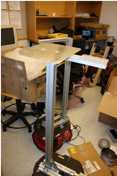
Figure 30: Top plate and PTU base plate on top beam
